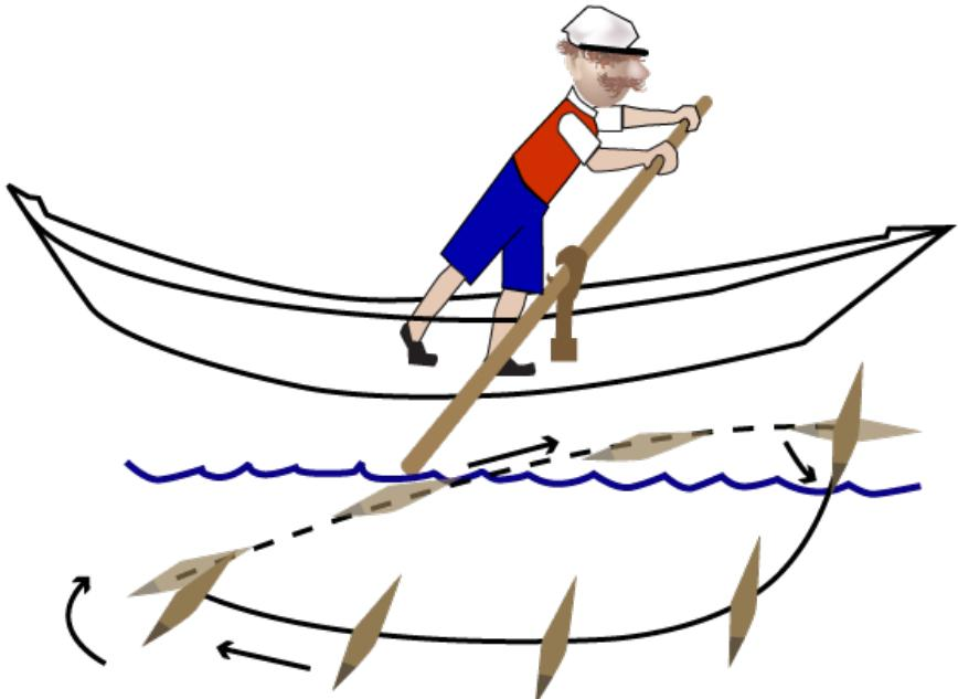
**En:** Forward stroke. Boat is pushed forward and to the left (port).
